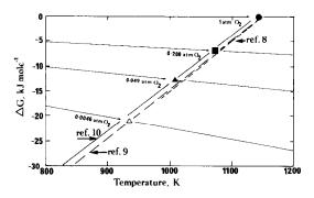
FIG. 2. Pourbaix-Ellingham diagram for the formation of PdO.  $\rightarrow$ ,  $RT \ln(P_{O2})^{1/2}$  versus temperature;  $\bigoplus$ ,  $\bigoplus$ , and  $\triangle$ , free energy equation, this work.
