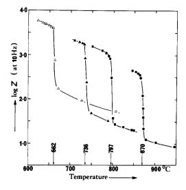
FIG. 1. The impedance-temperature relation at 10 Hz for a Pd/YSZ/Pd cell at:  $\oplus$ , 1 atm;  $\blacksquare$ , 0.208 atm;  $\blacktriangle$ , 0.049 atm; and  $\triangle$ , 0.0046 atm.
